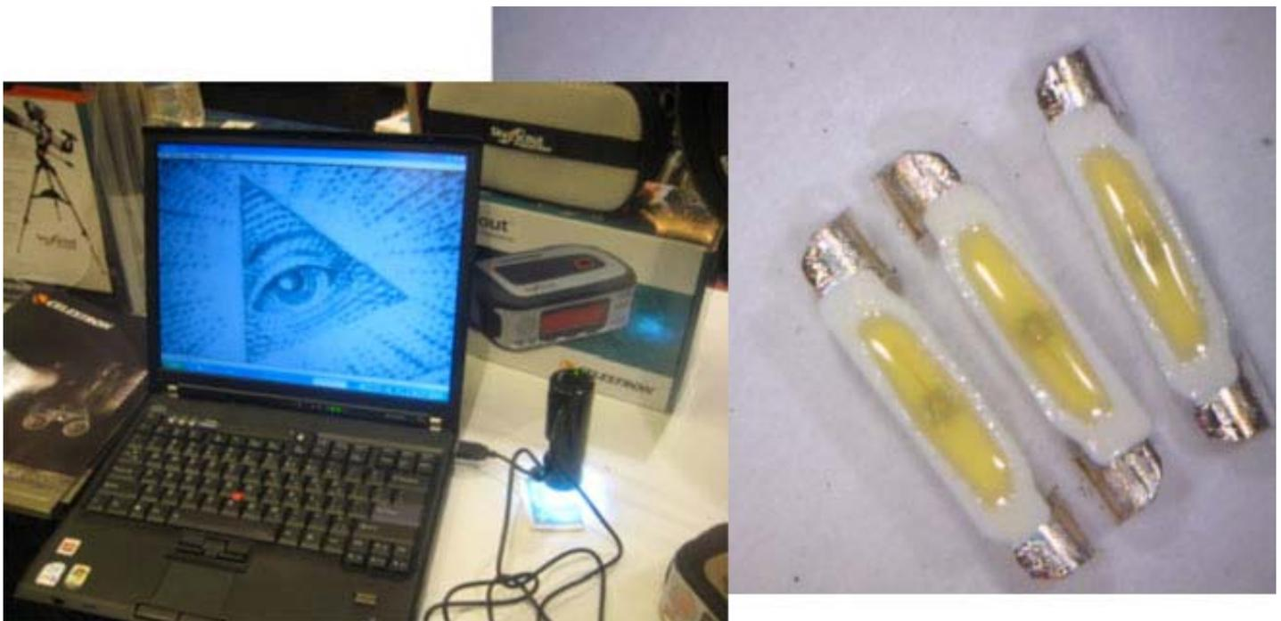
*Left: handheld, USB powered microscope and camera, Right: picture of LEDs taken in court*
